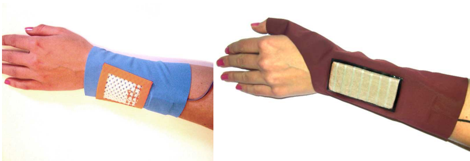
Figure 5: Left: Arm Band with Embroidered Circuitry Right: Arm Band with Pressure Sensitive Fabric and Extension for Bone Phone.
